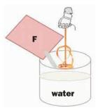
For mixing of single bags, it is acceptable to use a 25 litre steel pail as a mixing vessel, and mixing carried out using a slow speed electric drill (350/360 rpm) fitted with
